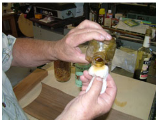
Using a manageable container like a small glass bottle or squeeze bottle, a small amount of shellac solution is applied to the dimpled center of the rubbing pad.
