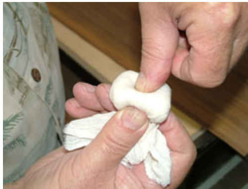
A dimple is formed in the middle of the tightly formed rubbing pad.
