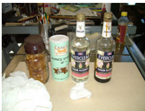
The basic ingredients and tools of the French polish process: shellac flakes, fine pumice powder, and unadulterated grain alcohol, with a fresh rubbing pad.
