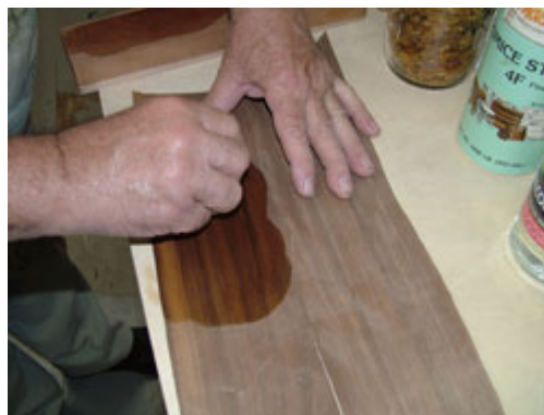
After only a few coats of shellac, the wood begins to take on a lustrous glow.
