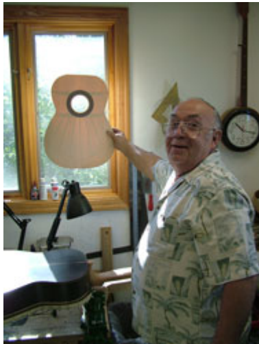
Light shows through a properly thinned and braced soundboard. Markle uses this damaged component in his lectures and demonstrations of luthiery technique.
