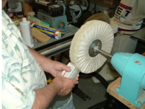
"Loading" the buffing wheel with Menzerna polishing compound.
